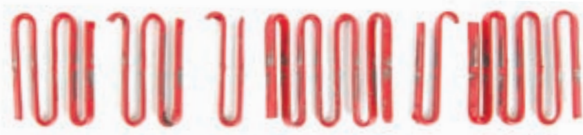
Dodge grid element after 70,000 cycles
