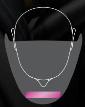
A flat lens in a slim helmet means the lens can't be wide.
