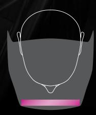
Expanded field of view with a flat lens requires a wider helmet.
