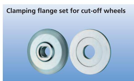
Special flange dia. 76 mm of tool steel for drive spindles M14 or 5/8". Increases lateral stability and improves power transmission on cut-off wheels.
